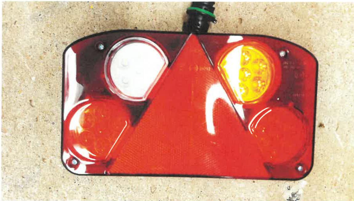
Lampa LED marka: Horpol, typu: LZD 2506/ADR/0,3M/AMP7, wariant: LZD 2506/ADR/0,3M/AMP7 LED lamp, make: Horpol, type: LZD 2506/ADR/0,3M/AMP7, variant: LZD 2506/ADR/0,3M/AMP7
